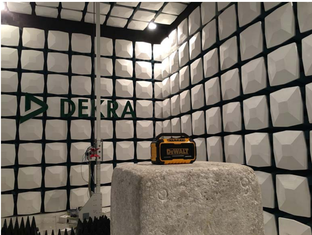
Description: Radiated Emission Test Setup for 1~18GHz
