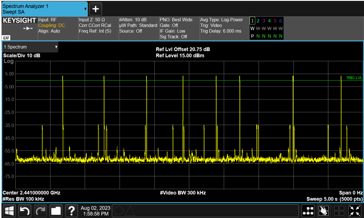
Figure 27: \pi/4 DQPSK Transmitter 5-Second Evaluation (Hopping)
