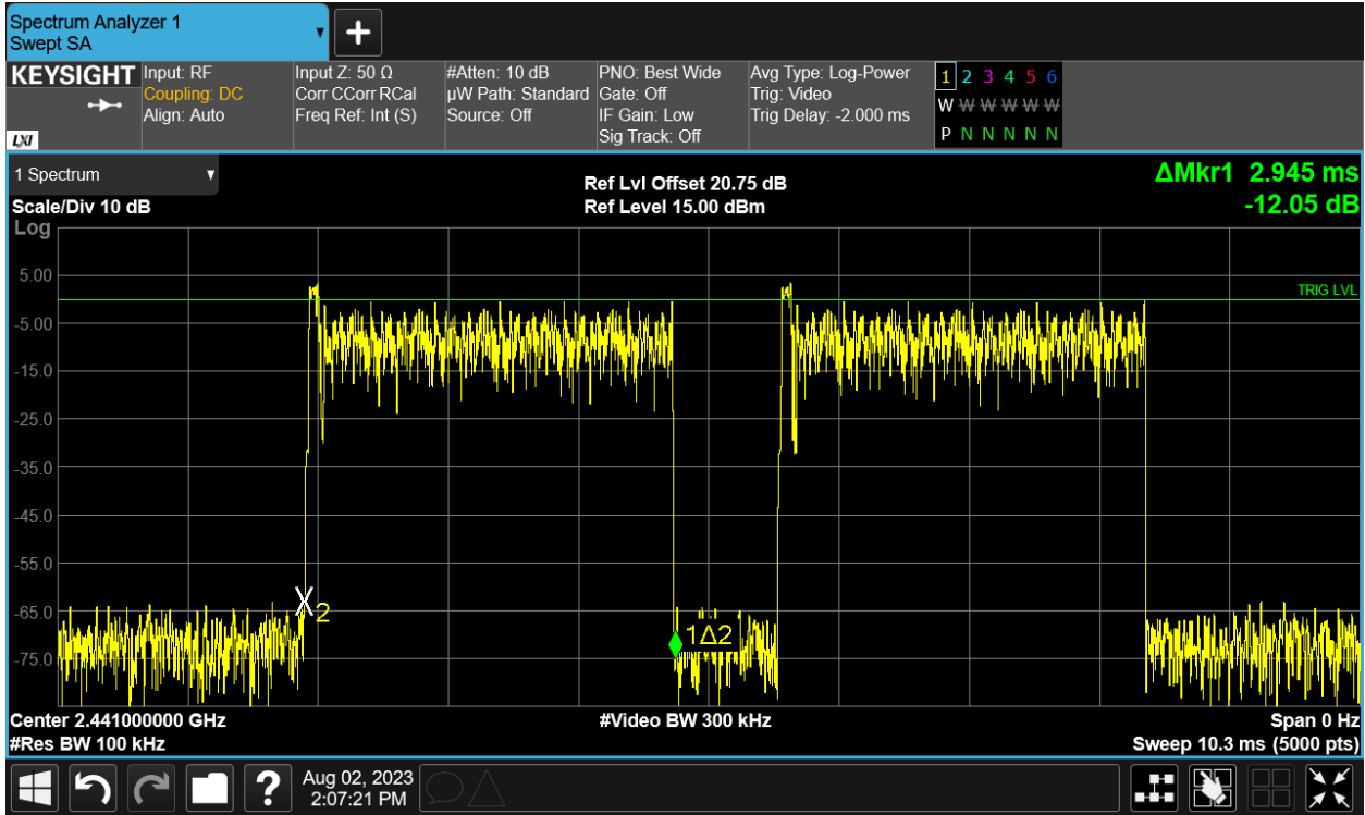
Figure 30: 8DPSK Transmitter Evaluation (Hopping) – Single Dwell Time
