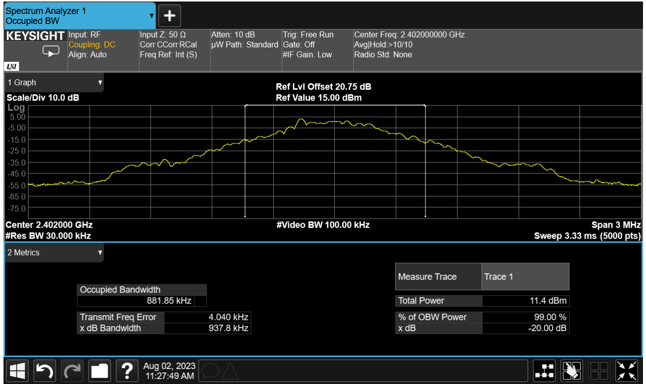
Figure 10: GFSK (1Mbps) – Low Channel, Occupied Bandwidth
