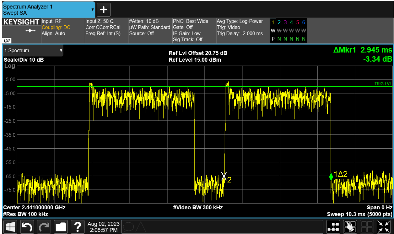
Figure 28: \pi/4 DQPSK Transmitter Evaluation (Hopping) – Single Dwell Time
