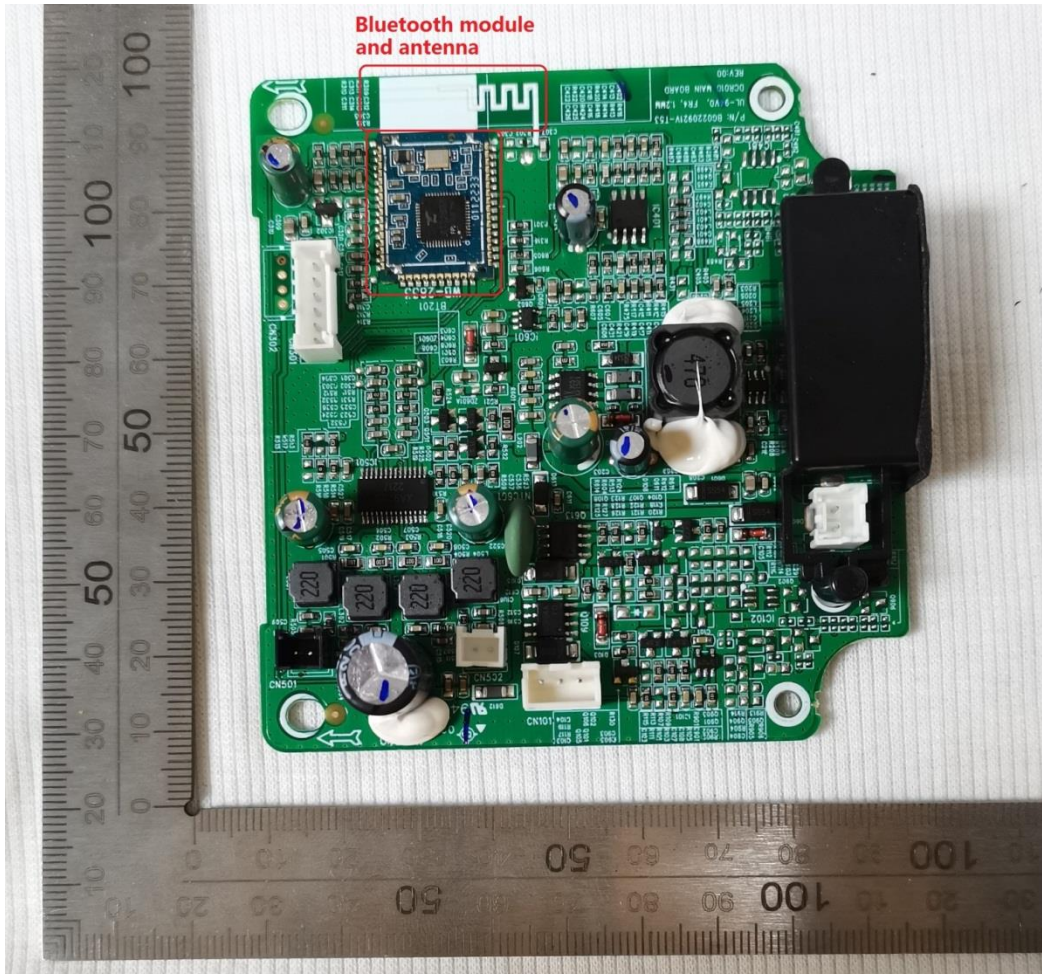
Figure 4: Complete board showing antenna location
