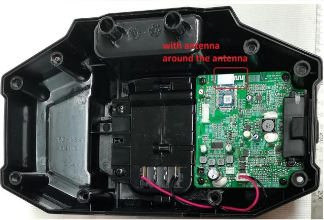
without shield around the antenna
