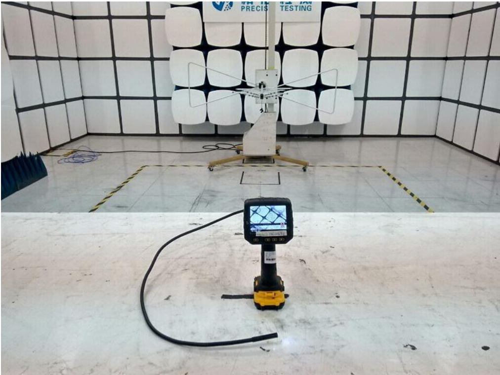
RADIATED EMISSION TEST SETUP ABOVE 1GHz
