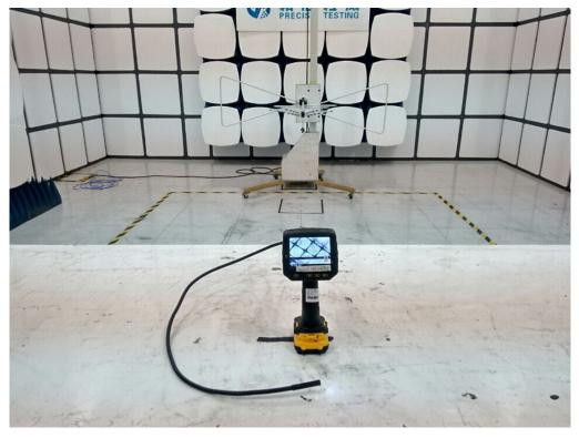
RADIATED EMISSION TEST SETUP ABOVE 1GHz
