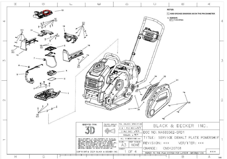
G2BLEM module mounting location circled in red above and below. The module is imbedded inside the enclosure where the tool battery is mounted.
