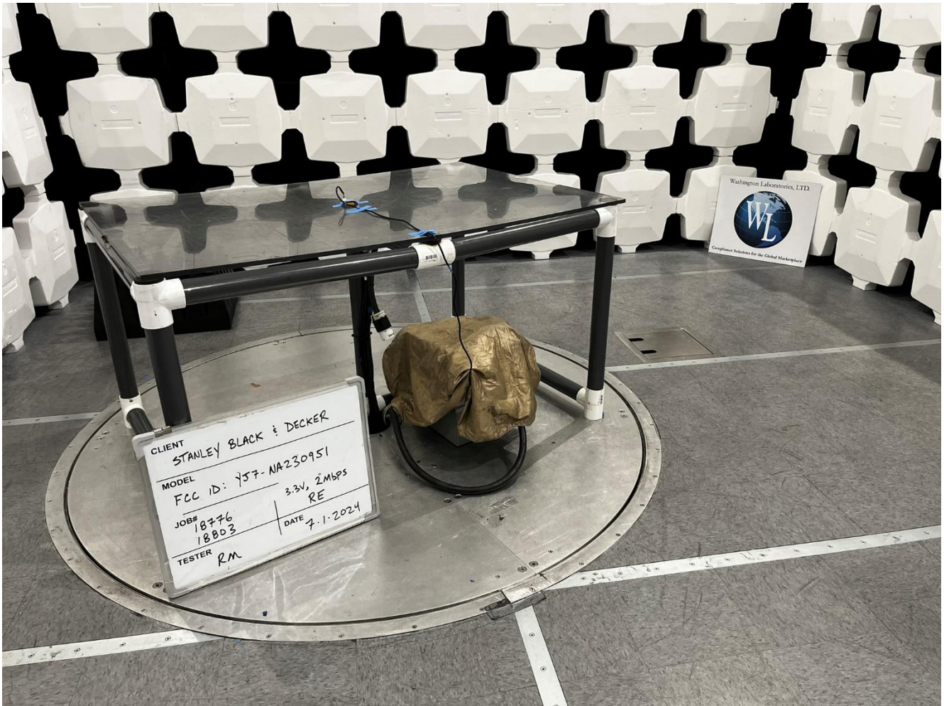
3-meter Radiated Emission, Rear View #1 (30M-1GHz)
