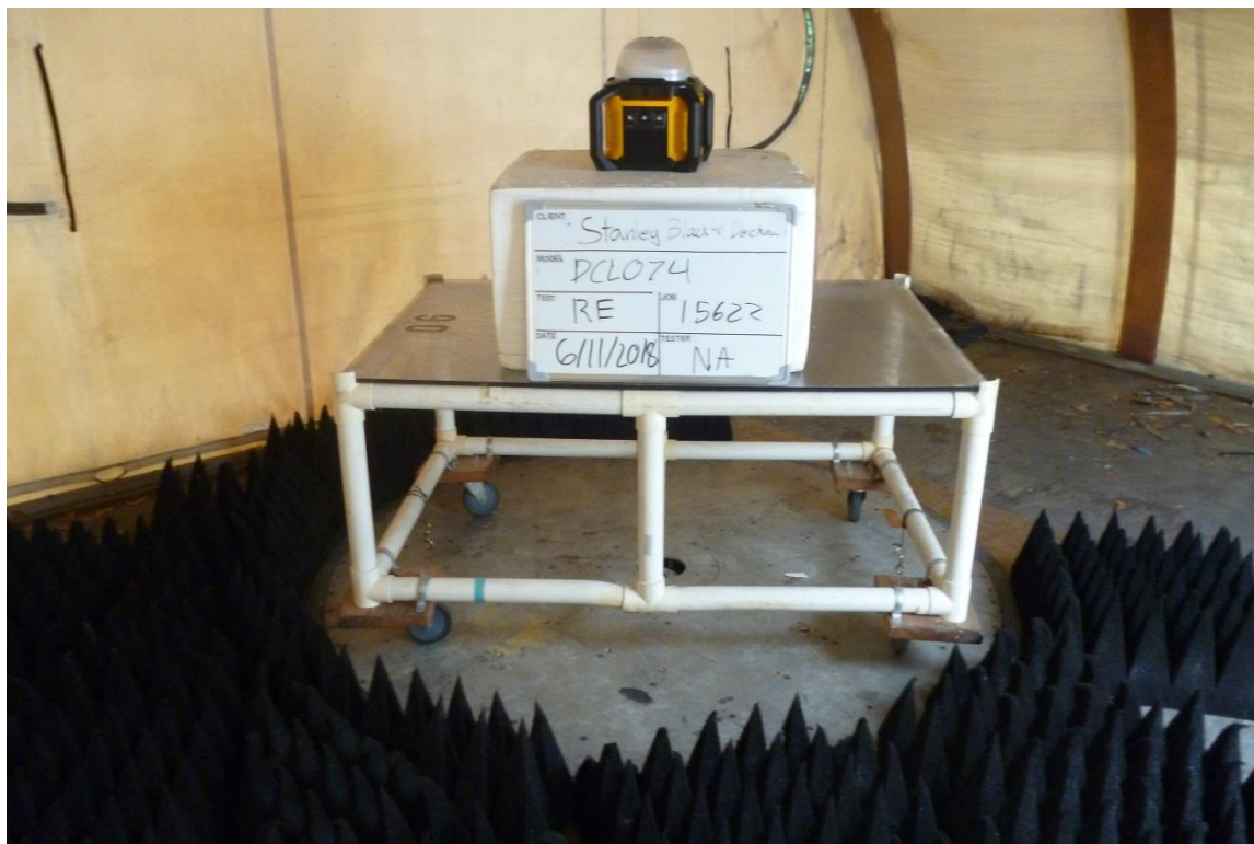
Photograph 4: Radiated Emissions Test Setup
