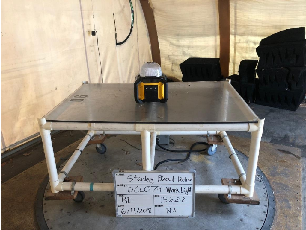
Photograph 2: Radiated Emissions Test Setup
