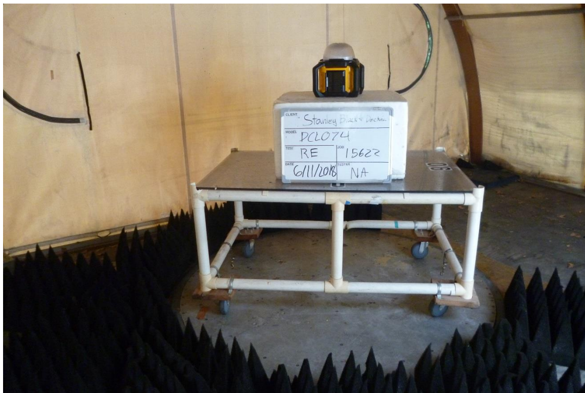
Photograph 5: Radiated Emissions Test Setup
