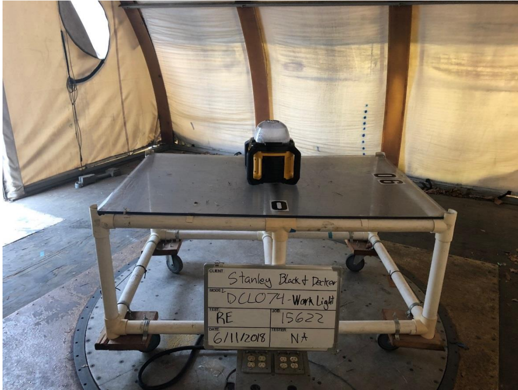
Photograph 3: Radiated Emissions Test Setup
