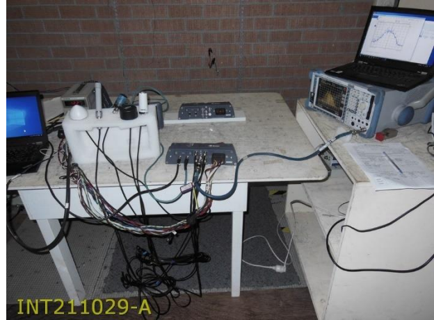
Conducted RF Test Bench
