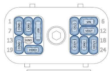
CONNECTIONS TO THE IVU PLUS ARE MADE USING DEUTSCH DRC26-24SA
