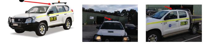
For the GPS to work accurately the Node must have clear line of sight to the sky. Obstructions such as machine structure, work roof or deep pit may affect the accuracy or operation of the GPS.
