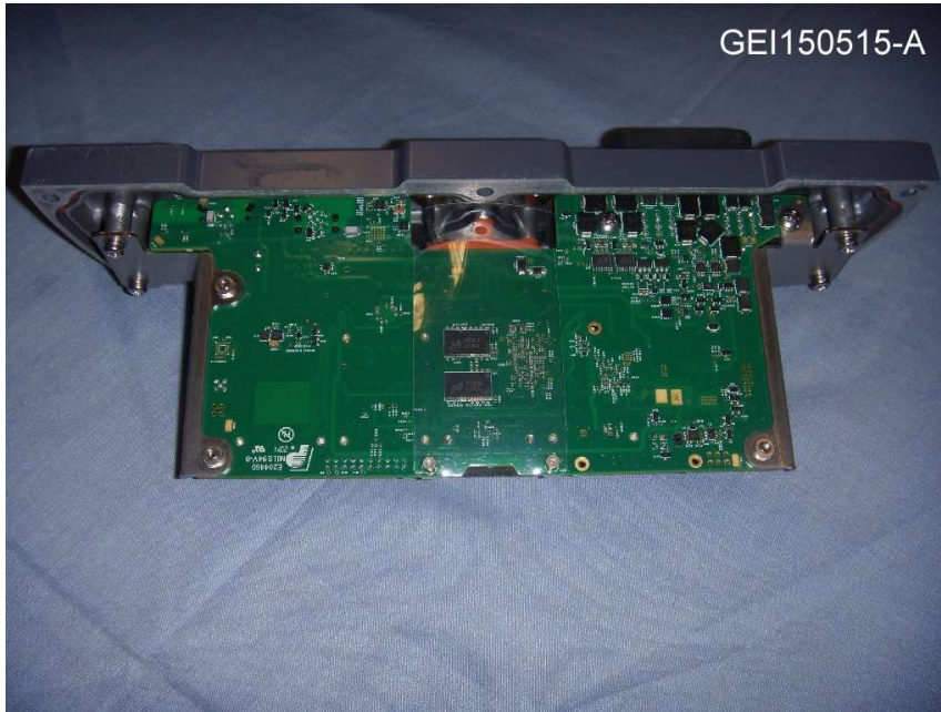
PROD0847-2 – Assembled Chassis Bottom
