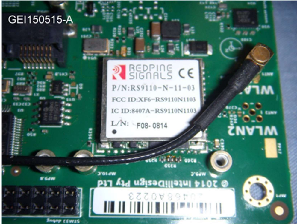
PROD0847-2 - WLAN Transceiver (on Main Board)
