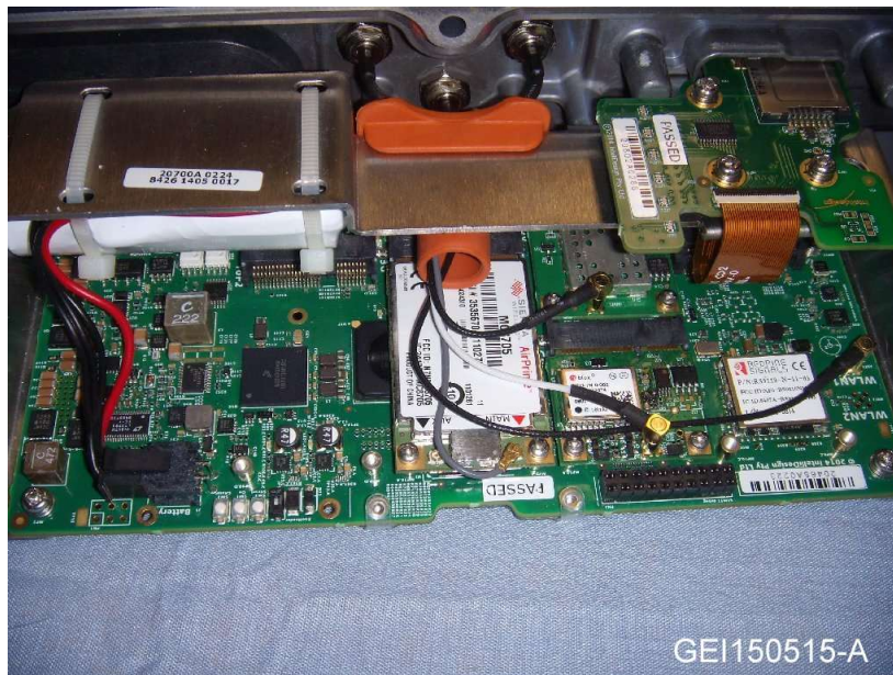
PROD0847-2 – Assembled Chassis Top (without Frame)
