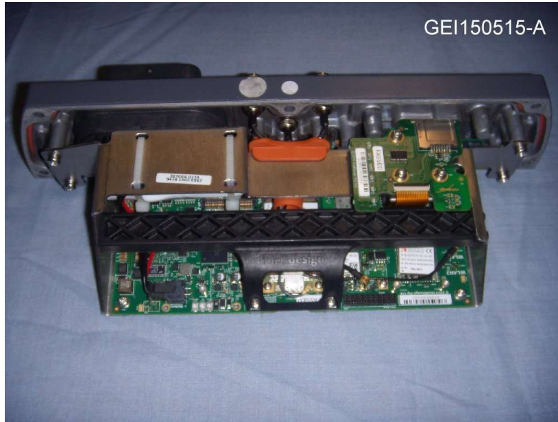
PROD0847-2 – Assembled Chassis Top (with Frame)
