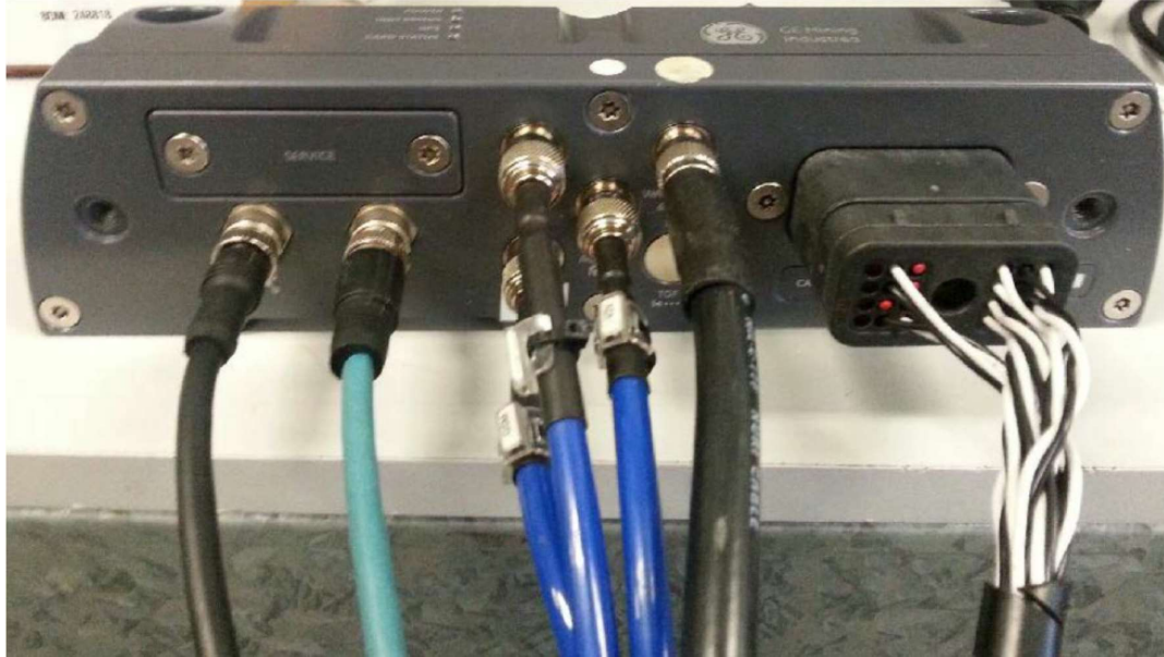
PROD0842-2 Cable Connections (There is no GSM antenna connected to this model)
