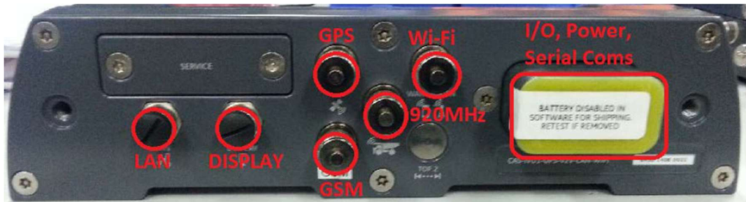
PROD0842-2 – Ports (GSM port is removed for this model)
