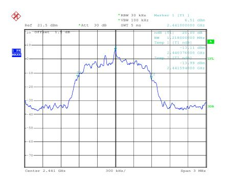
Test mode: π/4DQPSK Test channel: Highest
