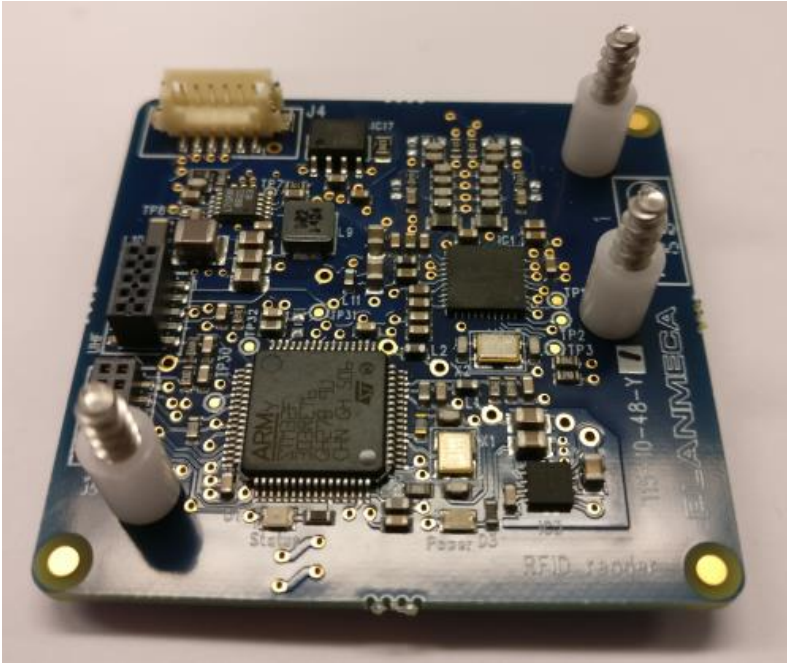
Picture 4: Spacers installed.
