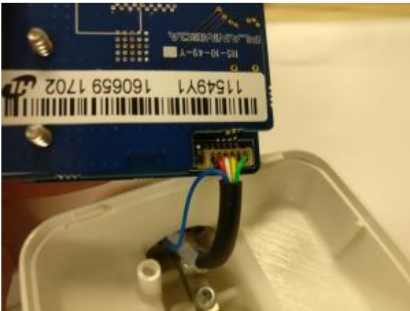
Picture 6: Cable assembled.
