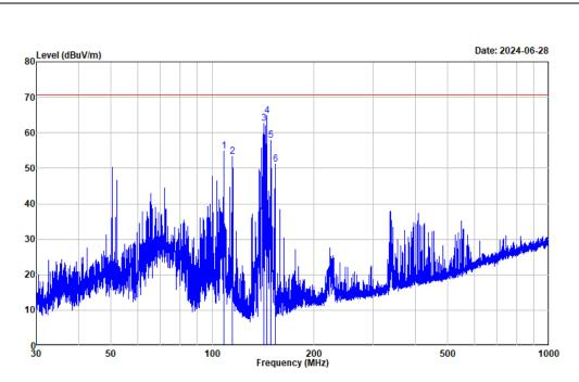
Project No. : 2405U32700E Test Mode : Microwave Test Voltage : AC 120V/60Hz
