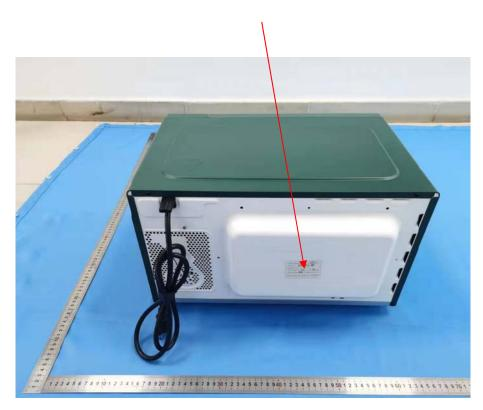
The label shown shall be permanently affixed at a conspicuous location on the device and be readily visible to the time purchase (Labeling requirements per 2.295)
