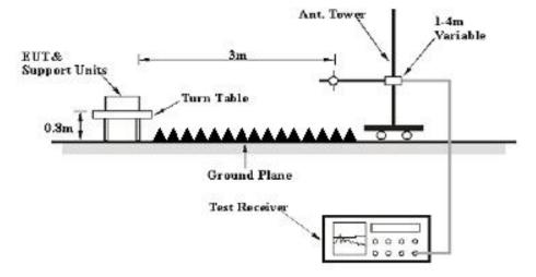
The radiated emission were performed in the 3 meters chamber test site, using the setup accordance with the FCC MP-5. The specification used was the FCC part 18 limits.
