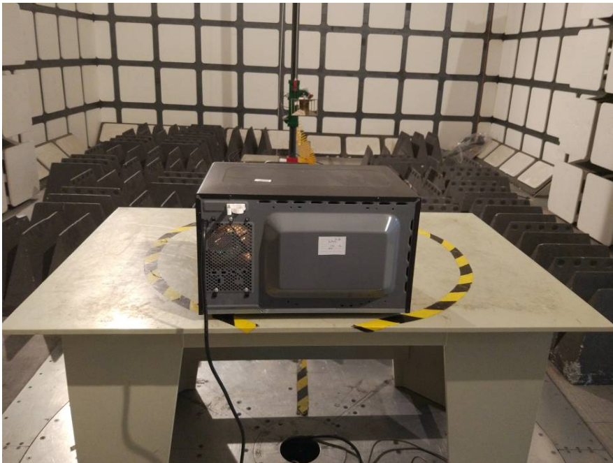
Radiated Emissions - Rear View (Above 1 GHz)
