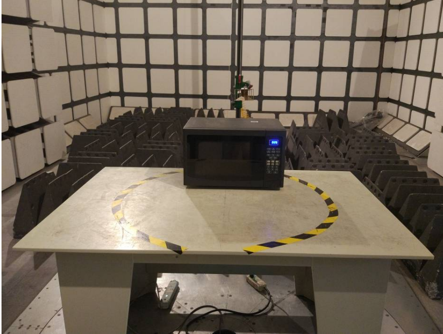
Radiated Emissions - Front View (Above 1 GHz)
