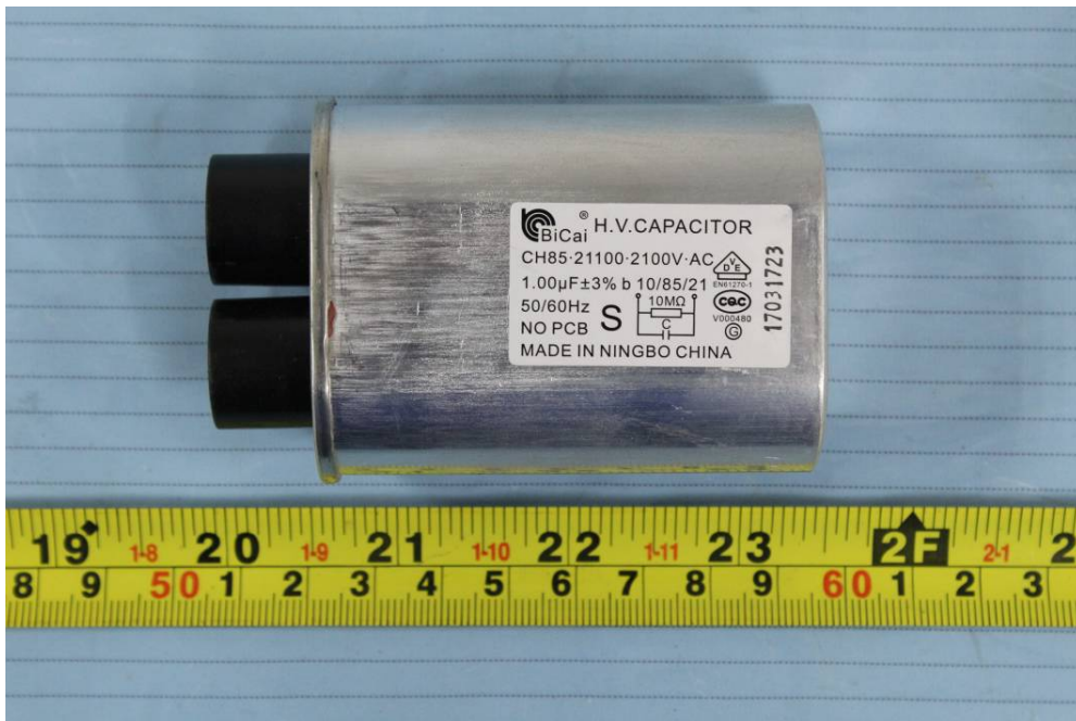
EUT –H.V. CAPACITOR View
