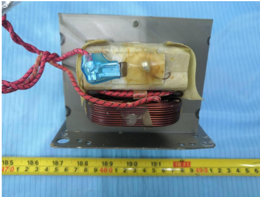
EUT – Transformer Top View
