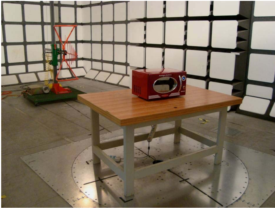
Radiated Emissions - Rear View (30 MHz-1 GHz)
