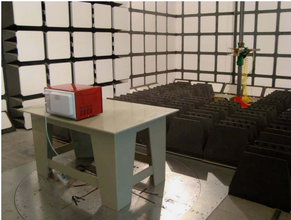
Radiated Emissions - Rear View (Above 1 GHz)
