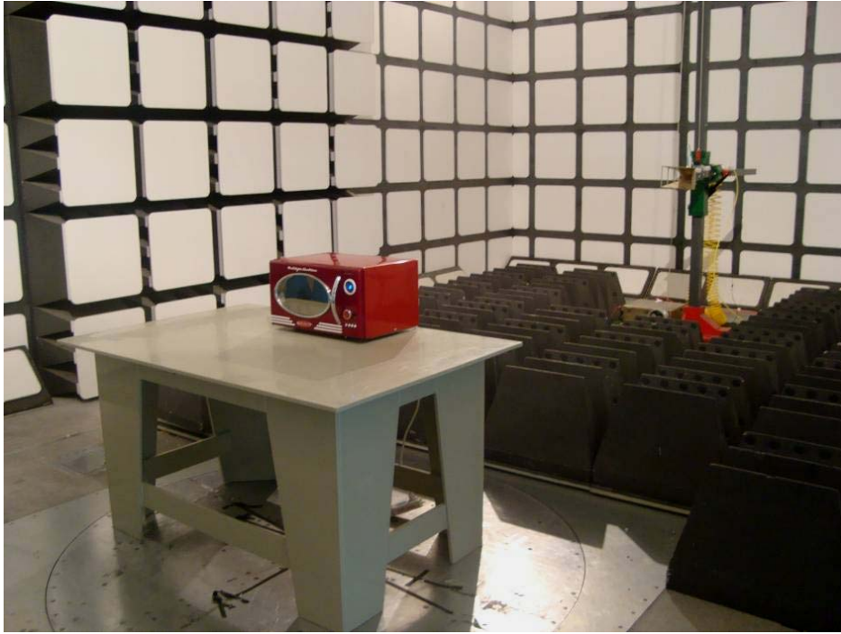
Radiated Emissions - Rear View (Above 1 GHz)
