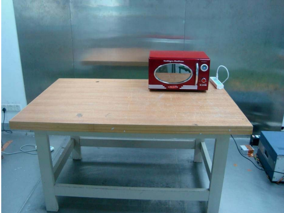
AC Line Conducted Emissions - Side View
