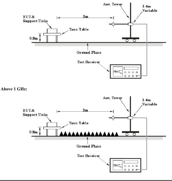
The radiated emission tests were performed in the 3 meters chamber test site, using the setup accordance with the FCC MP - 5. The specification used was the FCC part 18 limits.
