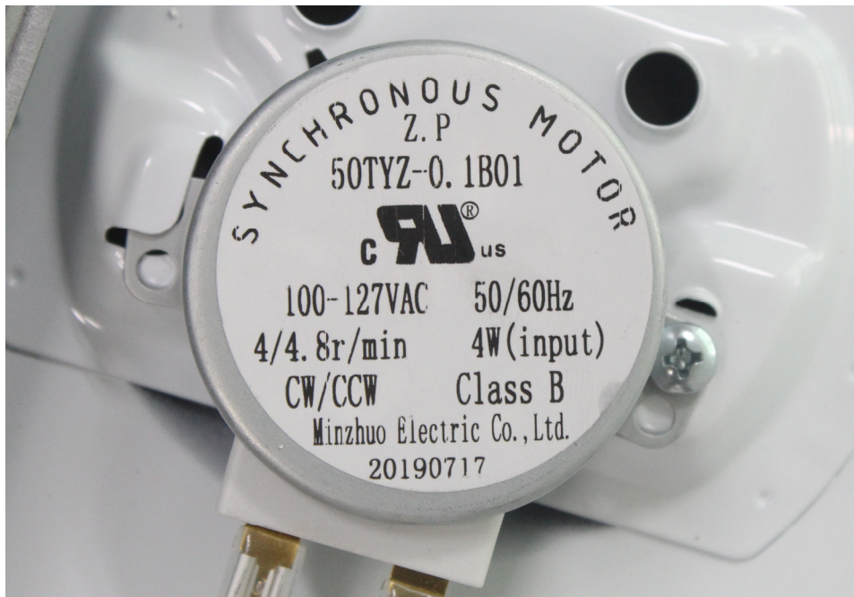
EUT – Synchronous Motor View
