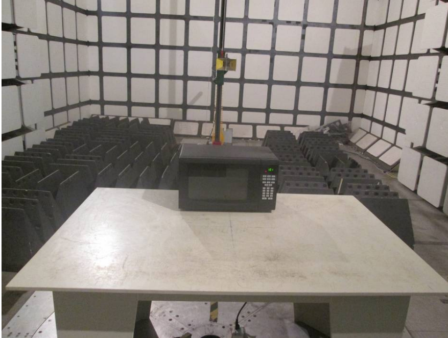
Radiated Emissions - Front View (Above 1 GHz)
