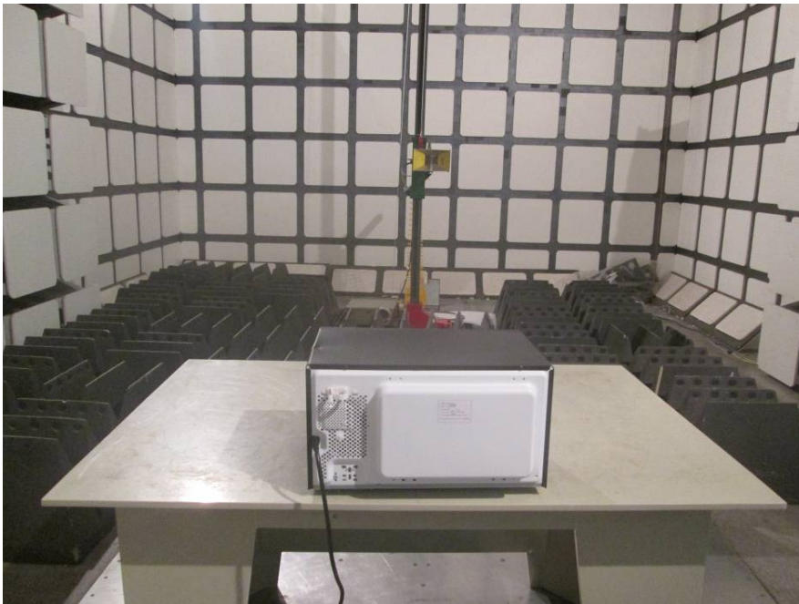
Radiated Emissions - Rear View (Above 1 GHz)
