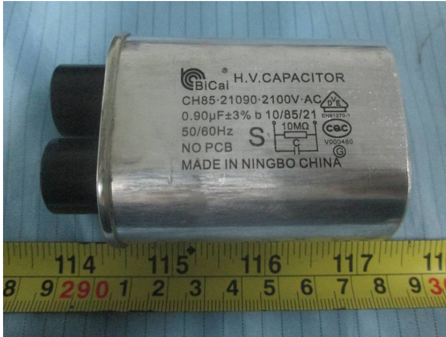
EUT – H.V. Capacitor View
