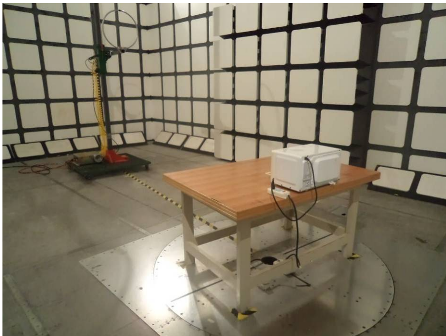
Radiated Emissions - Rear View (9 kHz – 30 MHz)
