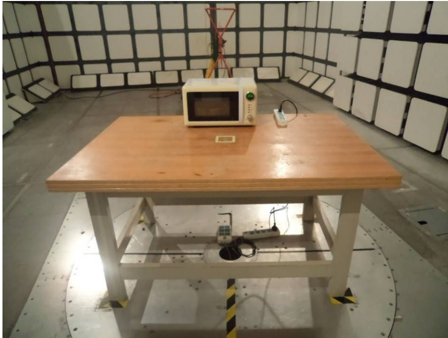
Radiated Emissions - Front View (30 MHz – 1 GHz)
