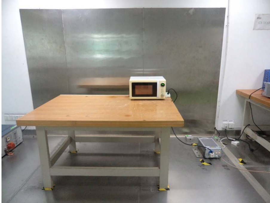
Conduction Emissions - Front View
