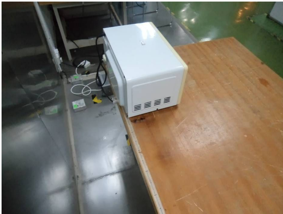
Conduction Emissions - Side View
