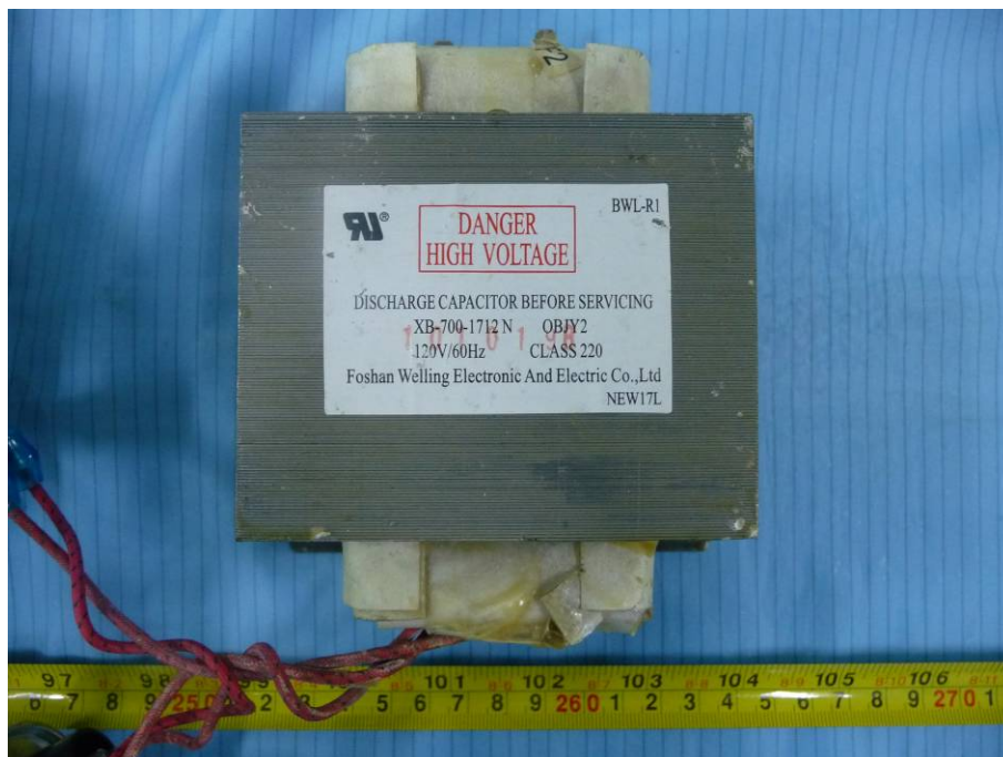
EUT – Power Transformer Top View
