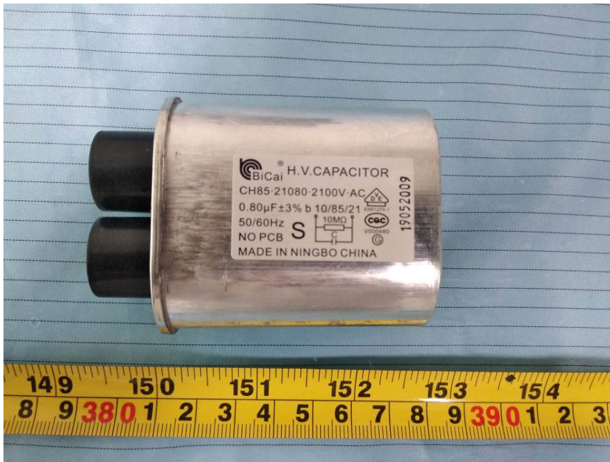
EUT – H.V. Capacitor Front View
