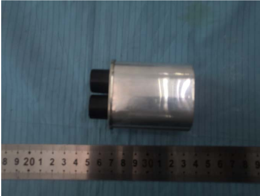
EUT – H.V. CAPACITOR Rear View
