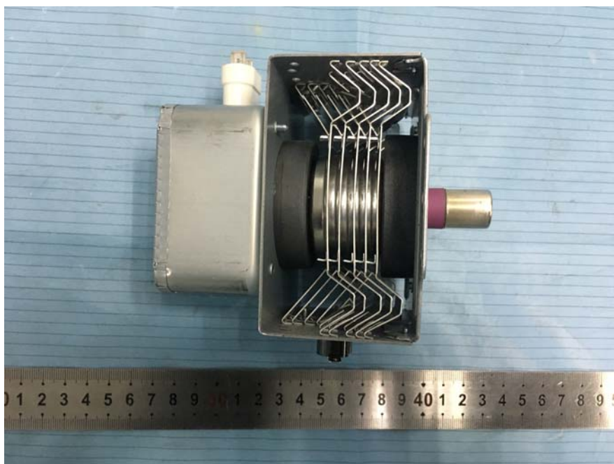
EUT – Magnetron Rear View (Type 2)
