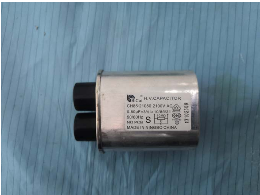
EUT – H.V. CAPACITOR Label View
