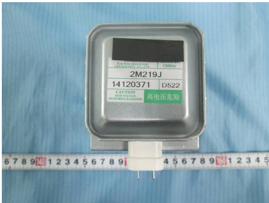
EUT – Magnetron Top View
