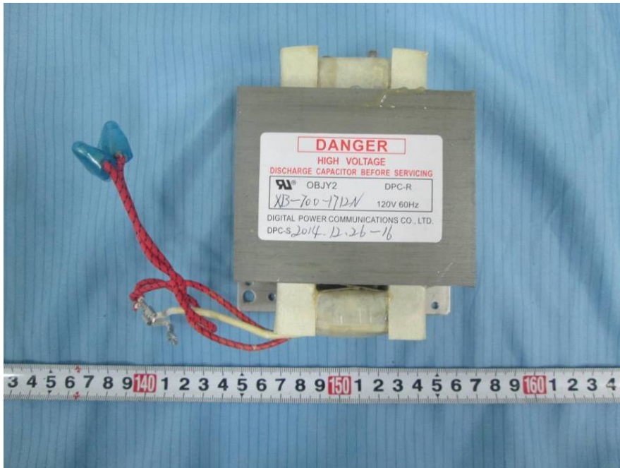
EUT – Transformer Top View
