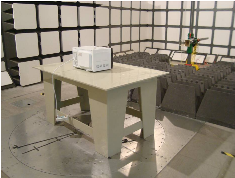
Radiated Emissions - Rear View (Above 1 GHz)
