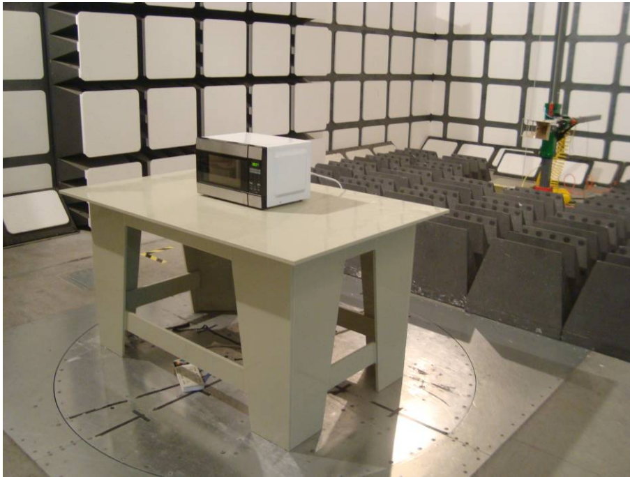
Radiated Emissions - Front View (Above 1 GHz)
