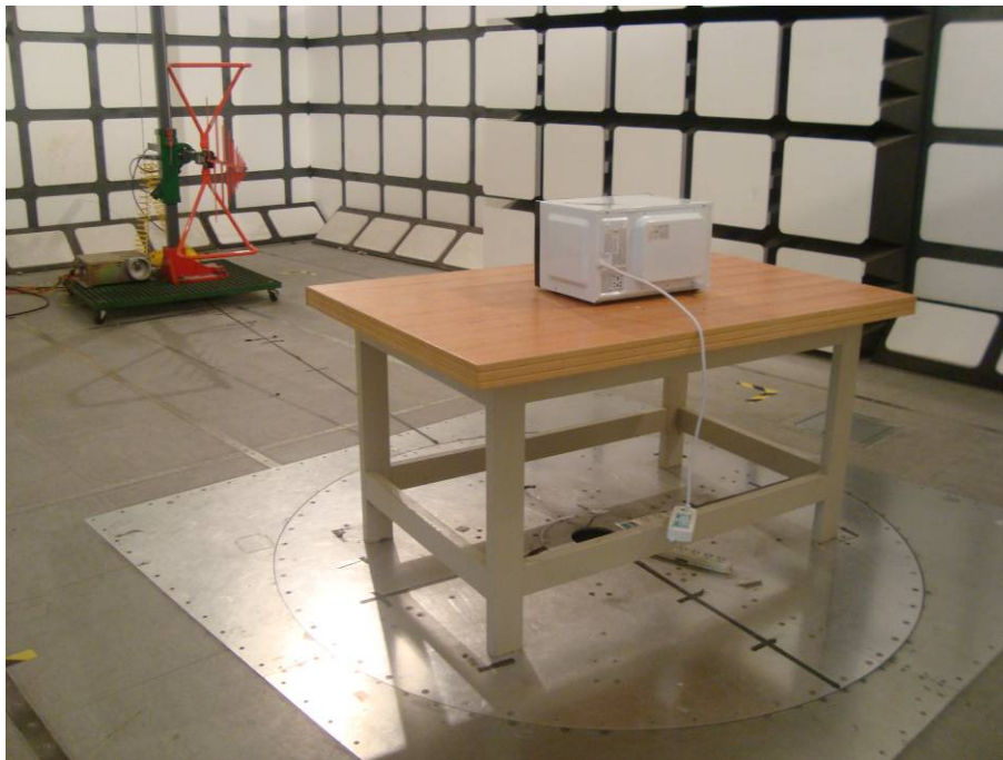
Radiated Emissions - Rear View (30 MHz-1 GHz)
