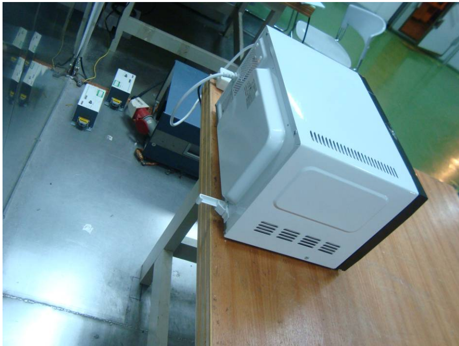
Conduction Emissions - Side View
