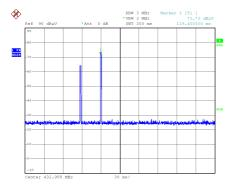
The transmission duration of one complete pulse train is 1.84ms.
