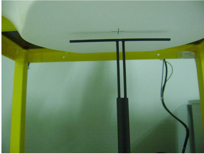
Setup Photo of Dipole Antenna
