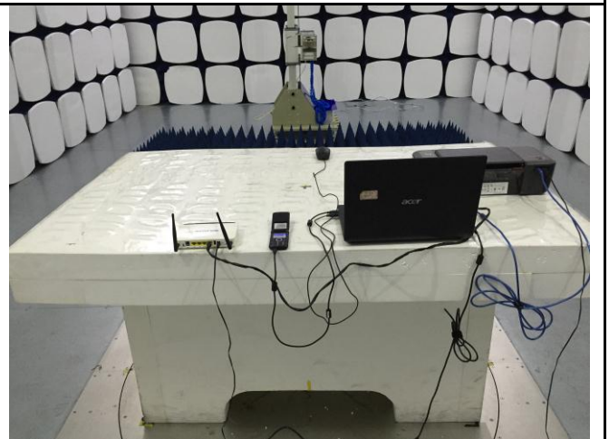
Radiated Emissions Test Setup Above 1GHz
