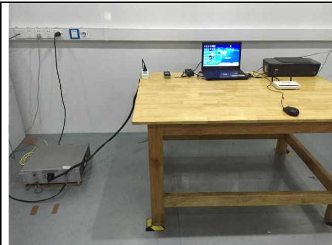
Conducted Emissions Test Setup – Front View
