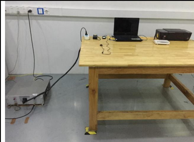
Conducted Emissions Test Setup – Front View
