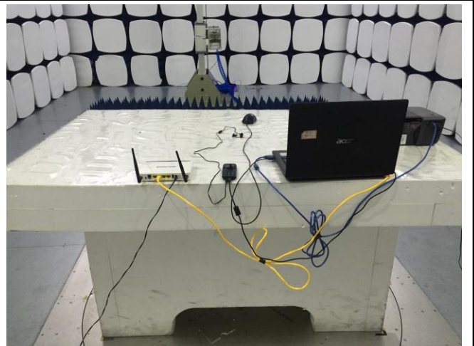
Radiated Emissions Test Setup Above 1GHz
