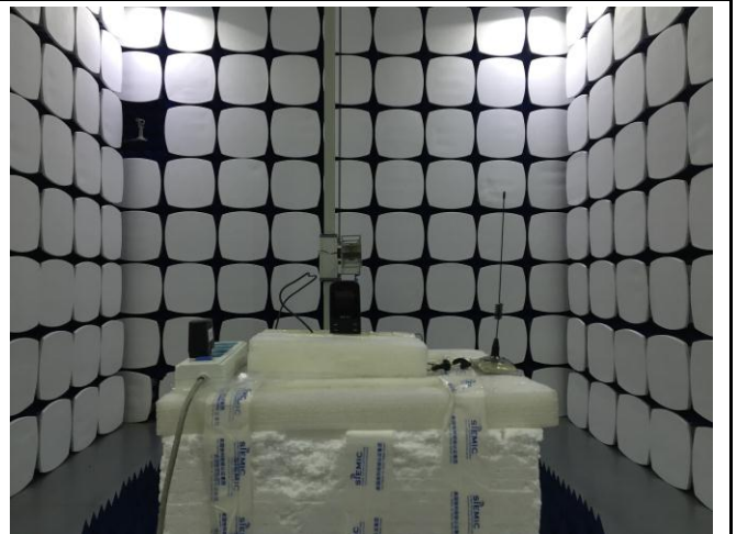
Radiated Spurious Emissions Test Setup Above 1GHz
