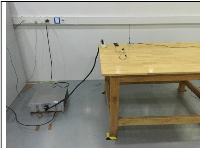
Conducted Emissions Test Setup Front View
