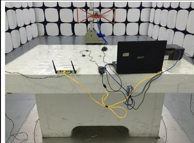
Radiated Emissions Test Setup Below 1GHz
