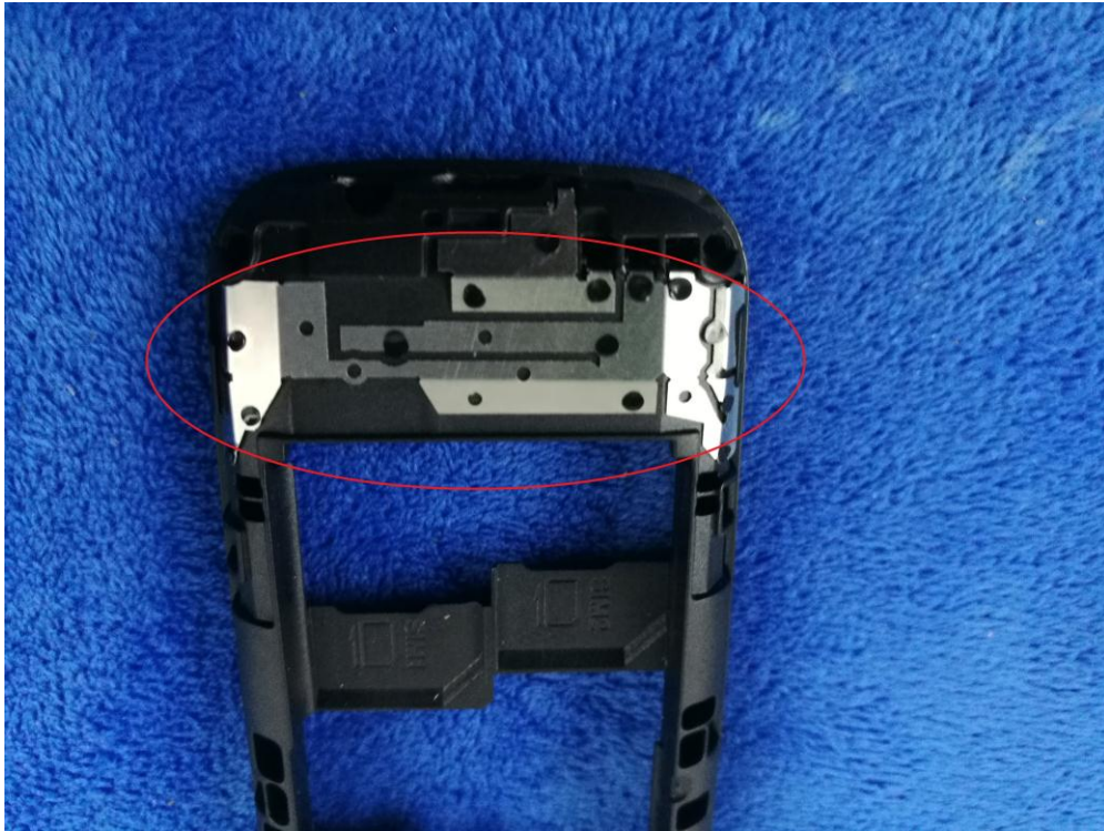
GSM/PCS Antenna View
