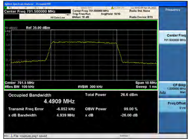
Band12 / 5MHz / Mid CH / 16QAM
