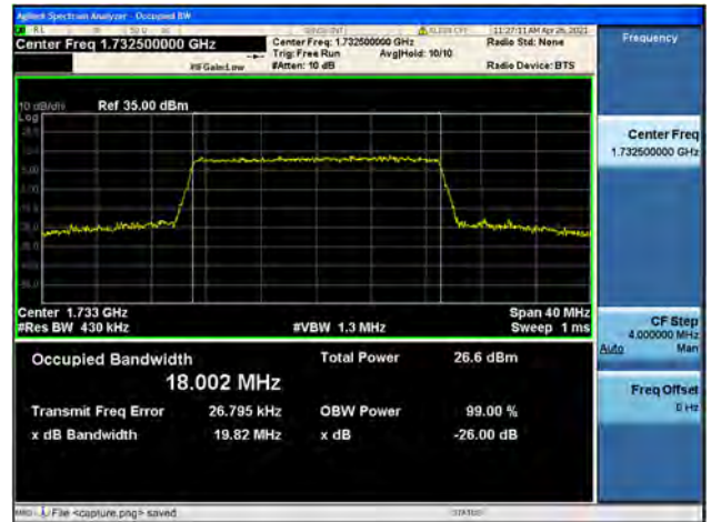
Band4 / 20MHz / High CH / 16QAM
