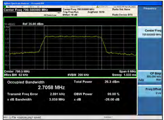
Band12 / 3MHz / Mid CH / 16QAM
