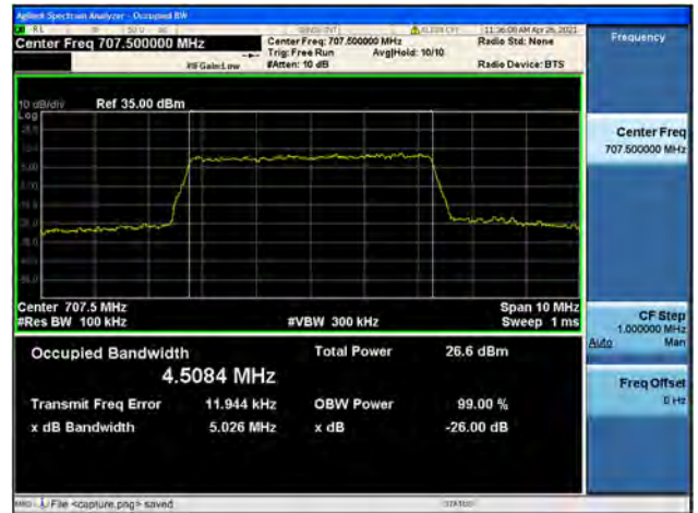
Band12 / 5MHz / High CH / 16QAM
