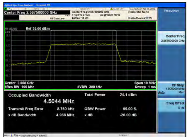
Band7 / 5MHz / High CH / 16QAM
