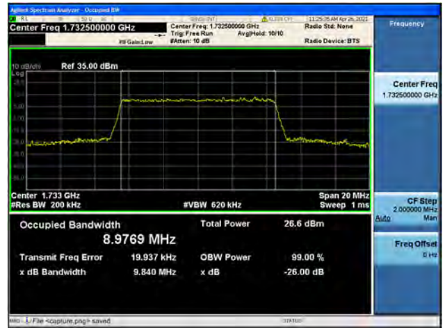
Band4 / 10MHz / High CH / 16QAM
