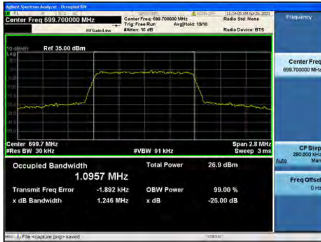
Band12 / 1.4MHz / Mid CH / QPSK
