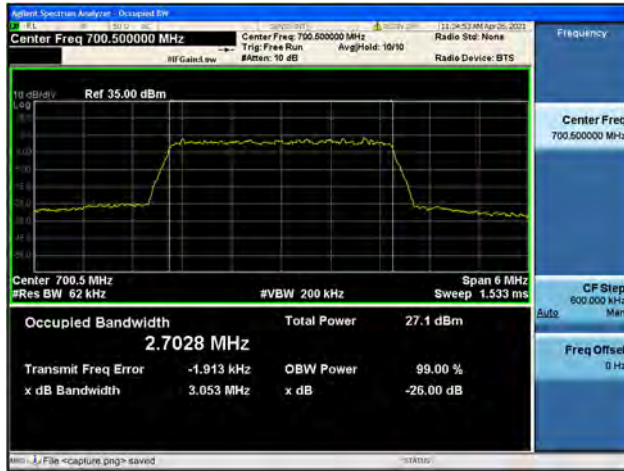
Band12 / 3MHz / Mid CH / QPSK
