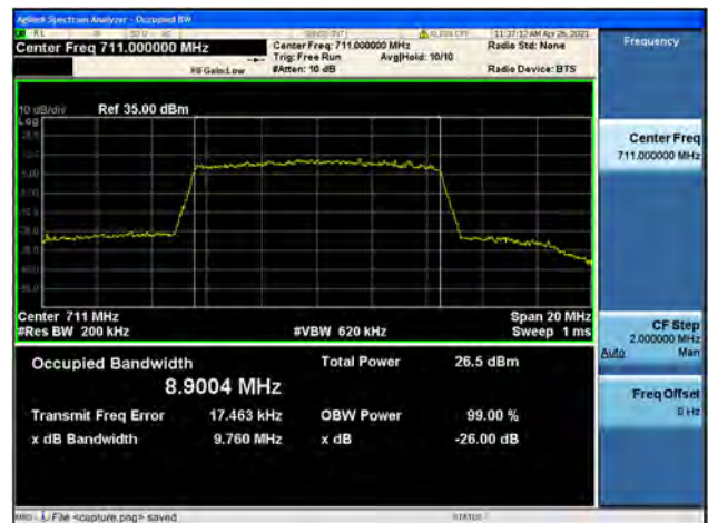
Band12 / 10MHz / High CH / 16QAM
