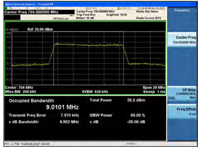
Band12 / 10MHz / Mid CH / 16QAM
