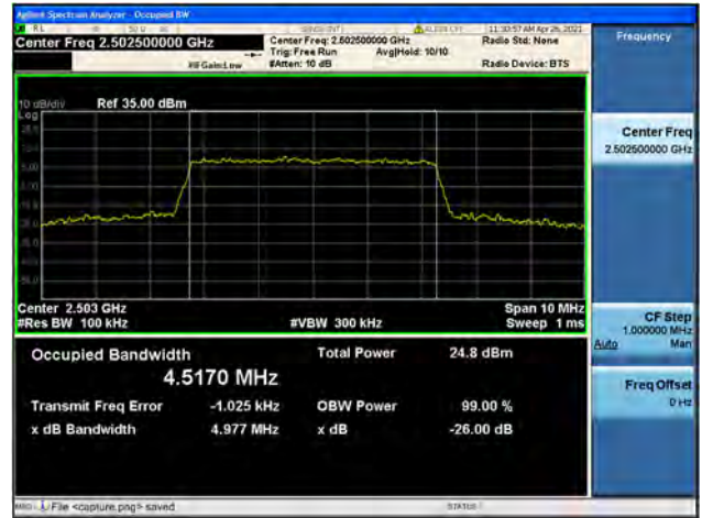
Band7 / 5MHz / Mid CH / 16QAM
