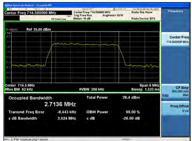
Band12 / 3MHz / High CH / 16QAM
