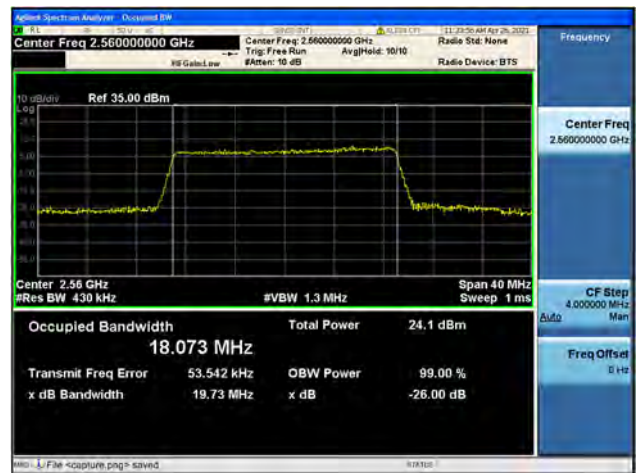
Band7 / 20MHz / High CH / 16QAM
