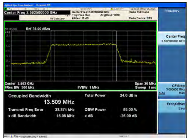
Band7 / 15MHz / High CH / 16QAM
