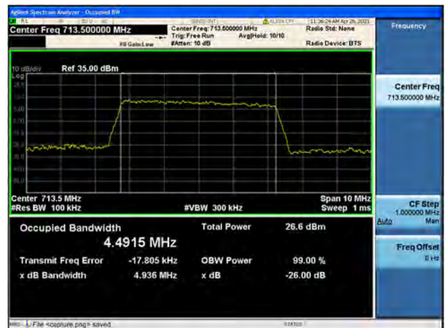
Band12 / 5MHz / High CH / 16QAM
