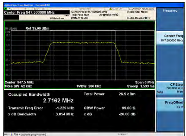
Band5 / 3MHz / High CH / 16QAM
