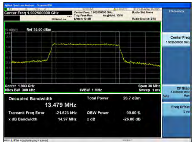
Band2 / 15MHz / High CH / 16QAM
