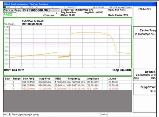
B12 / 3MHz / Low CH / QPSK / FULL RB
