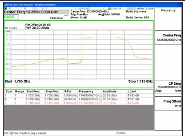
B66 / 3MHz / Low CH / QPSK / FULL RB
