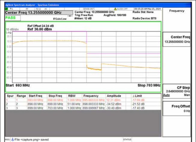
B71 / 5MHz / High CH / QPSK / FULL RB
