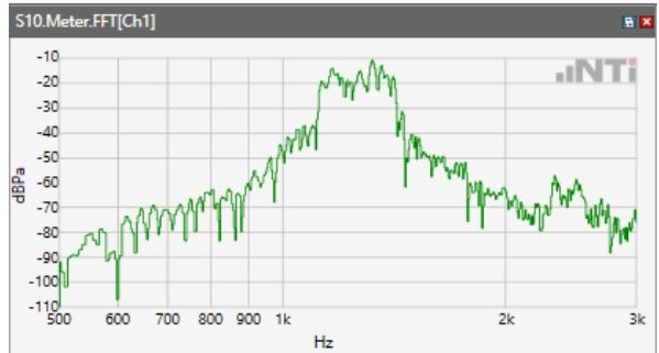
ANSI/TIA 5050-2018 \ 8N HAC OFF \ WB 23.85 kbps\ 5.2 Receive path – distortion and noise\WCDMA Band II
