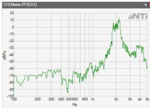
ANSI/TIA 5050-2018 \ 8N HAC OFF \ WB 23.85 kbps\ 5.2 Receive path – distortion and noise\WLAN 5.5GHz
