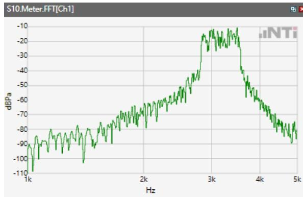
ANSI/TIA 5050-2018 \ 8N HAC OFF \ NB 12.2kbps\ 5.2 Receive path – distortion and noise\WLAN 5.5 GHz
