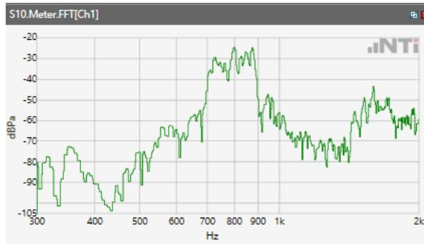
ANSI/TIA 5050-2018 \ 8N HAC OFF \ NB 12.2kbps\ 5.2 Receive path – distortion and noise\WLAN 5.5 GHz
