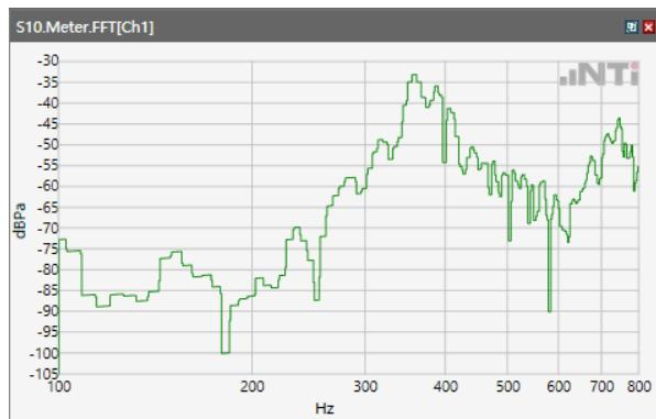
ANSI/TIA 5050-2018 \ 8N HAC OFF \ WB 23.85 kbps\ 5.2 Receive path – distortion and noise\WLAN 5.8GHz
