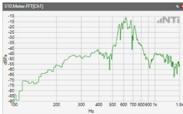
ANSI/TIA 5050-2018 \ 8N HAC OFF \ WB 23.85 kbps\ 5.2 Receive path – distortion and noise\WLAN 5.3GHz
