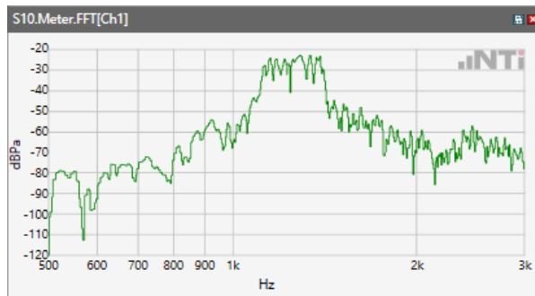
ANSI/TIA 5050-2018 \ 8N HAC OFF \ NB 12.2kbps\ 5.2 Receive path – distortion and noise\WLAN 5.5 GHz
