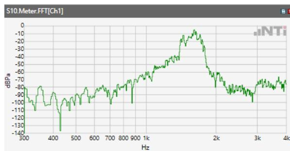
ANSI/TIA 5050-2018 \ 8N HAC OFF \ WB 23.85 kbps\ 5.2 Receive path – distortion and noise\LTE Band 12
