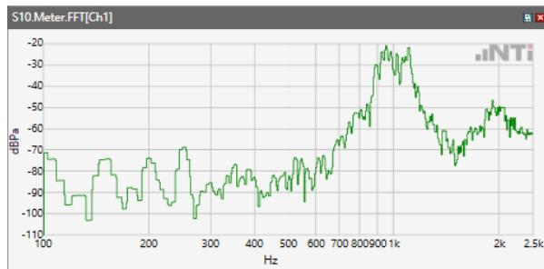
ANSI/TIA 5050-2018 \ 8N HAC OFF \ NB 12.2kbps\ 5.2 Receive path – distortion and noise\WLAN 5.2 GHz
