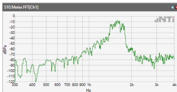
ANSI/TIA 5050-2018 \ 8N HAC OFF \ WB 23.85 kbps\ 5.2 Receive path – distortion and noise\WLAN 2.4GHz
