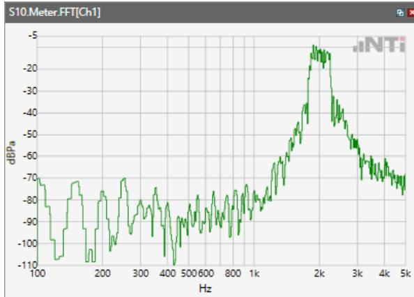
ANSI/TIA 5050-2018 \ 8N HAC OFF \ NB 12.2kbps\ 5.2 Receive path – distortion and noise\WLAN 5.5 GHz
