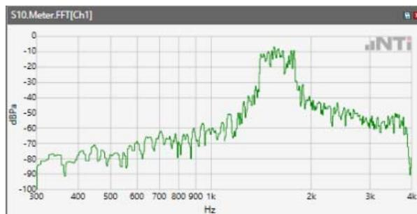
ANSI/TIA 5050-2018 \ 8N HAC OFF \ WB 23.85 kbps\ 5.2 Receive path – distortion and noise\WLAN 5.3GHz
