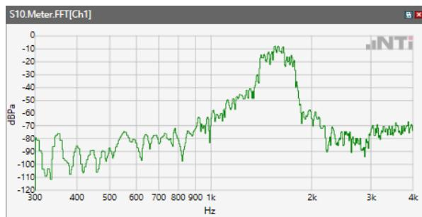
ANSI/TIA 5050-2018 \ 8N HAC OFF \ NB 12.2kbps\ 5.2 Receive path – distortion and noise\WCDMA Band V
