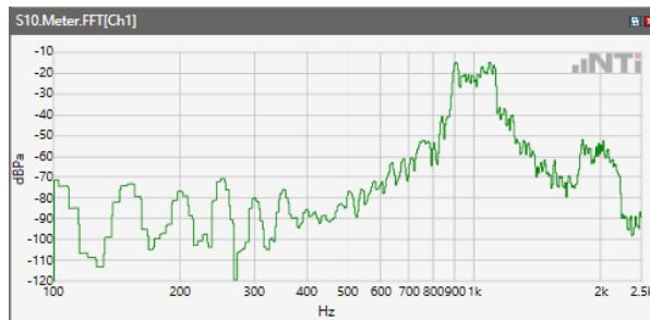
ANSI/TIA 5050-2018 \ 8N HAC OFF \ NB 12.2kbps\ 5.2 Receive path – distortion and noise\LTE Band 7
