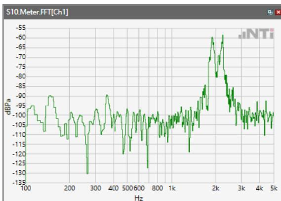
ANSI/TIA 5050-2018 \ 8N HAC OFF \ WB 23.85 kbps\ 5.2 Receive path – distortion and noise\WLAN 5.2GHz
