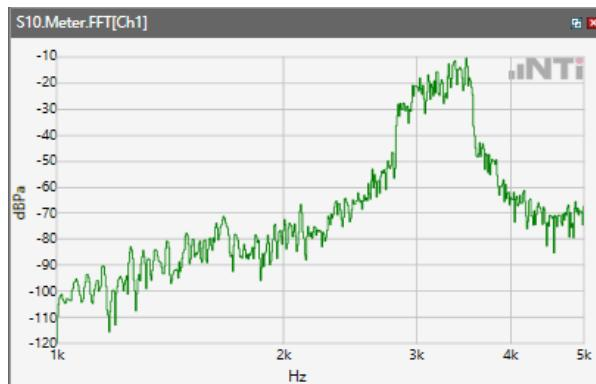
ANSI/TIA 5050-2018 \ 8N HAC OFF \ NB 12.2kbps\ 5.2 Receive path – distortion and noise\WCDMA Band II
