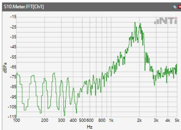
ANSI/TIA 5050-2018 \ 8N HAC OFF \ WB 23.85 kbps\ 5.2 Receive path – distortion and noise\LTE Band 71
