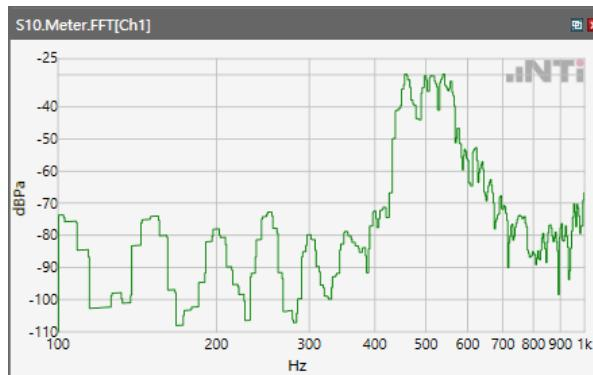
ANSI/TIA 5050-2018 \ 8N HAC OFF \ WB 23.85 kbps\ 5.2 Receive path – distortion and noise\WCDMA Band V
