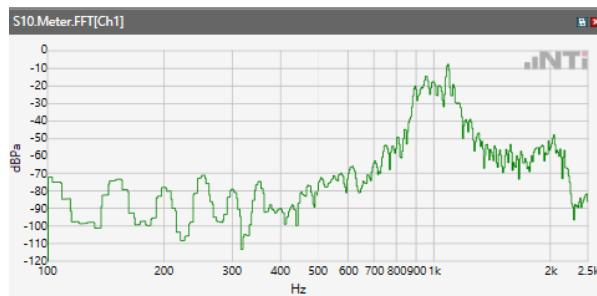
ANSI/TIA 5050-2018 \ 8N HAC OFF \ WB 23.85 kbps\ 5.2 Receive path – distortion and noise\LTE Band 7
