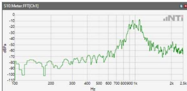
ANSI/TIA 5050-2018 \ 8N HAC OFF \ WB 23.85 kbps\ 5.2 Receive path – distortion and noise\WLAN 5.3GHz
