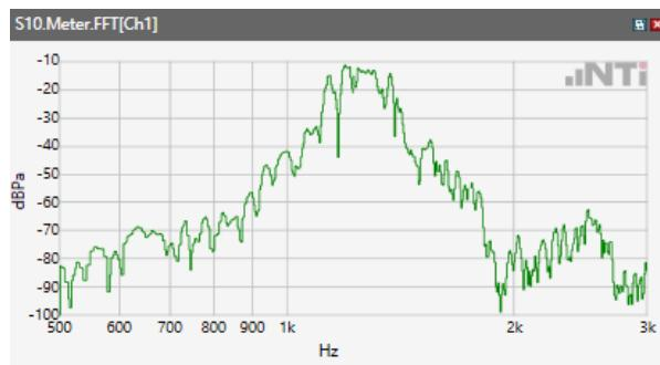
ANSI/TIA 5050-2018 \ 8N HAC OFF \ NB 12.2kbps\ 5.2 Receive path – distortion and noise\LTE Band 7
