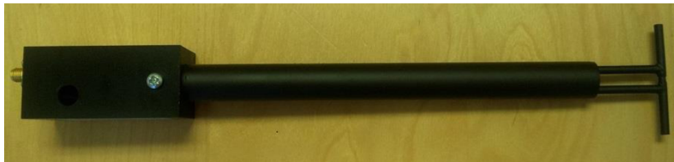
Figure 1 – MVG COMOSAR Validation Dipole
