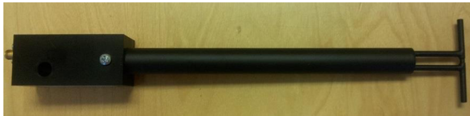
Figure 1 – MVG COMOSAR Validation Dipole
