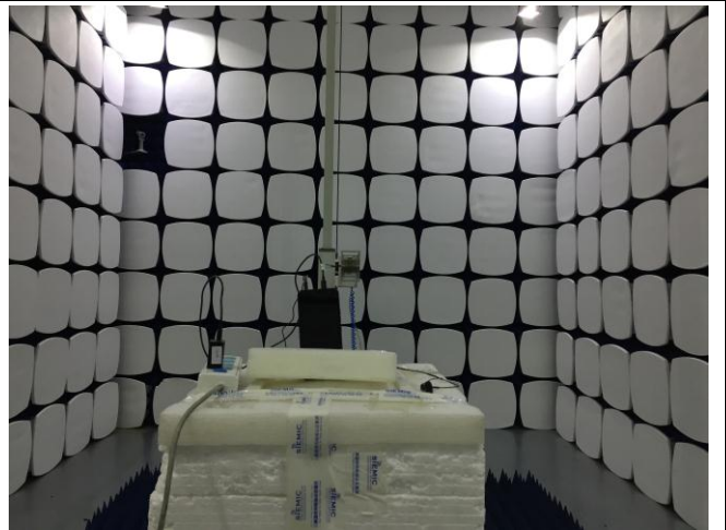
Radiated Spurious Emissions Test Setup Above 1GHz
