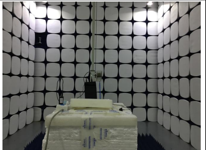
Radiated Spurious Emissions Test Setup Above 1GHz
