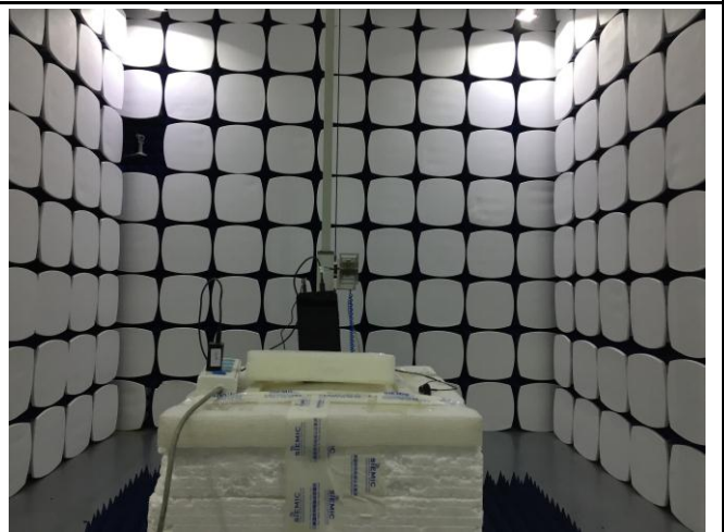
Radiated Spurious Emissions Test Setup Above 1GHz
