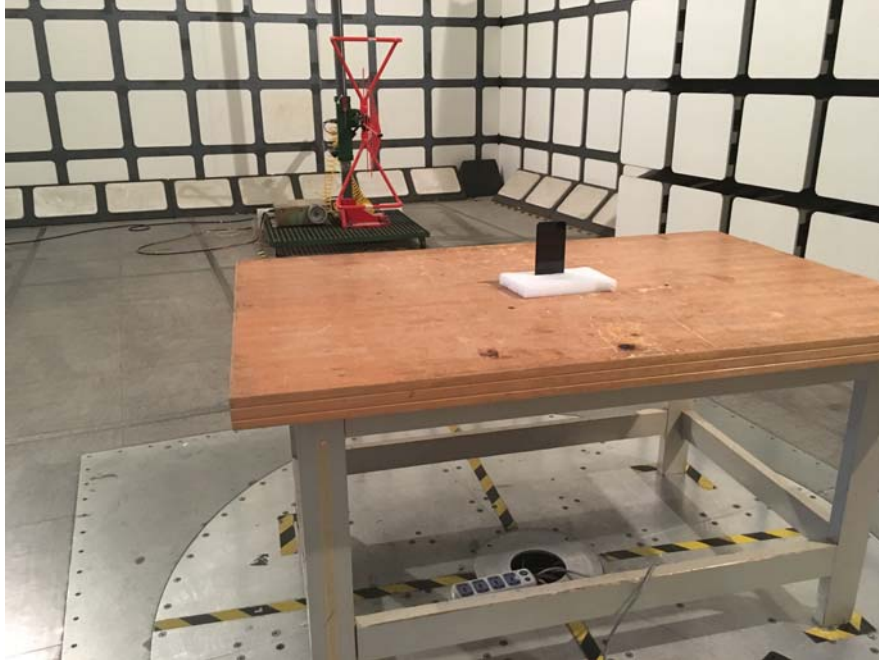
Radiated Emissions View (Below 1 GHz)
