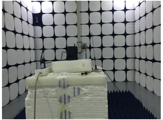
Radiated Spurious Emissions Test Setup Above 1GHz
