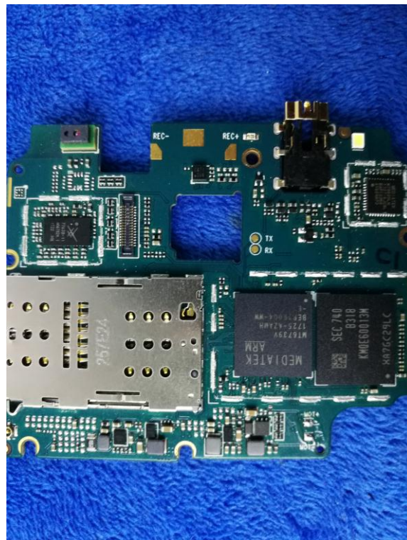
Mainboard without Shielding - Rear View
