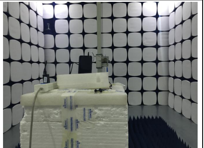
Radiated Spurious Emissions Test Setup Above 1GHz
